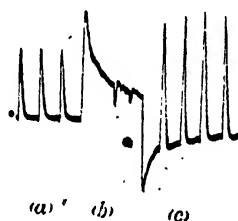
Fig. 77. Photographic record showing the effect of continuous stimulation in enhancing response (Pt). Each curve shows response (followed by recovery), the stimulus being kept constant throughout. The series of responses (a), enhanced to series (c) after continuous vibration (b).
